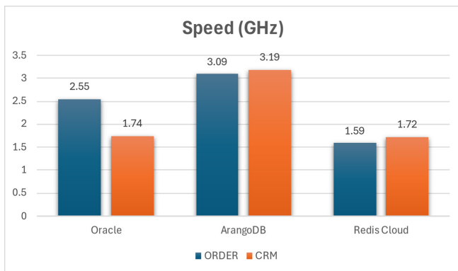
Figure 8: Speed Performance for Data Retrieval Across All Database Models.
